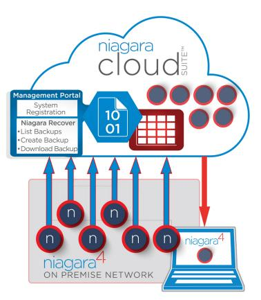
Subscribers select Niagara Instances to be backed up, either at the supervisory or field-JACE level. Storage efficiency is assured through Binary Large Object (BLOB) cloud architecture, with associated meta data maintained. Encrypted data is directly streamed to the Niagara Cloud account. Backups can be initiated programmatically and on-demand from a Niagara station. Subscribers can list backups and retrieve backups via the Management Portal.
