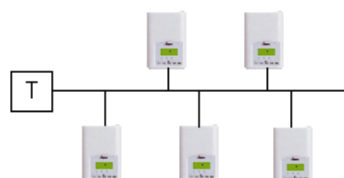
Figure 3.1 Singly Terminated Bus Topology
