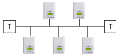
Figure 3.2 Doubly Terminated Bus Topology
